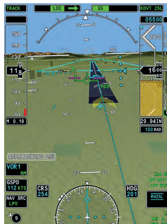
Right: Synthetic vision systems combine satellite signals with a database of pictures of the surrounding terrain
