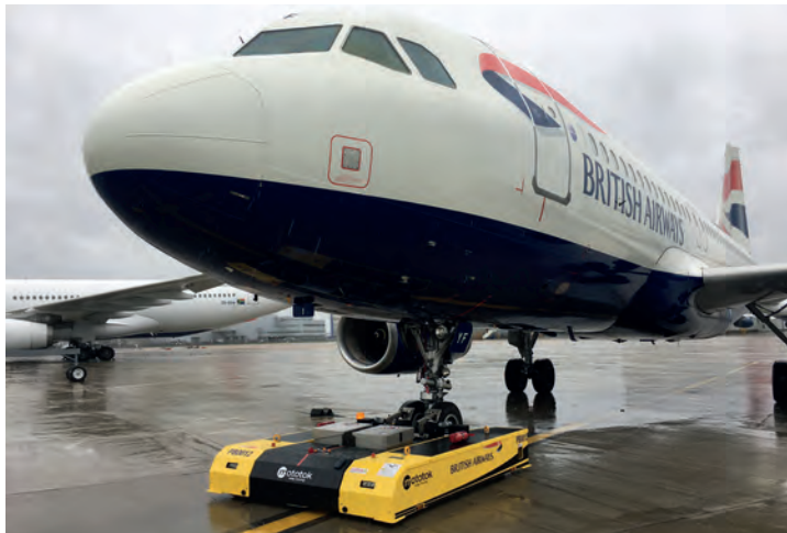
Above: The Spacer 8600 pushes back aircraft for British Airways' medium-haul flights
