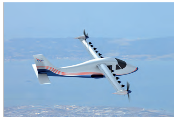
Above: Boeing's X-57 Maxwell experimental airplane has 14 electric motors integrated into a uniquely designed wing
